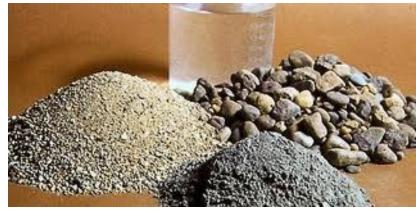
**CONCRETE** is a composite material that consists essentially a binding medium within which are embedded particles of aggregate
